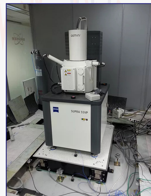
At installation, VEC custom tunes the DVIA-M control systems based on the data recorded during the site survey.
