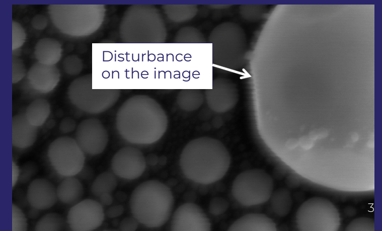
Figure 1: Vibration, magnetic fields, and acoustic noise can result in disturbance or edge noise on an electron microscope image.
