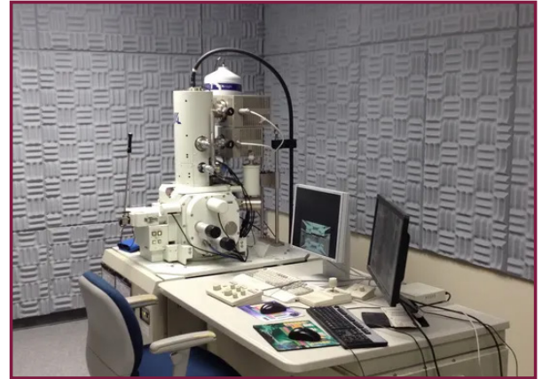
Acoustic panels on the walls provide noise reduction in electron microscopy labs.
