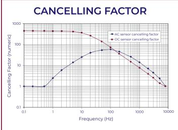
The SC24/DC+AC Sensor cancels fields from DC to 5k Hz, while the SC24/AC Sensor provides excellent cancellation of 60 Hz and its harmonics.
